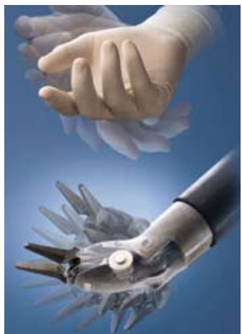
Hand of da Vinci robot (below) showing its greater dexterity compared with human hand.
